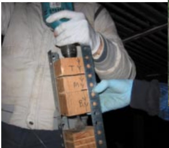
Harley White and Jacob White use an excellently devised jig to drill a 1 1/8" hole into the end of a 4x4
